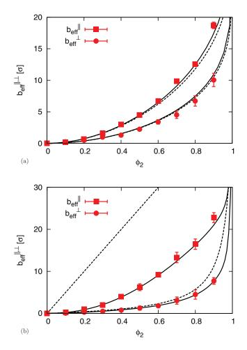
FIG. 6. The eigenvalues of the effective slip length tensor (symbols) as a function of  $\phi_2$ . Solid curves are theoretical values obtained by a numerical solution of Eqs. (19), (20) and (30), (31). Calculations were made for a pattern with  $L = b = 50\sigma$ , (a)  $H = 50\sigma$ . Dashed curves are calculated with Eqs. (22) and (38), (b)  $H = 10\sigma$ . Dashed curves are computed with Eqs. (21) and (35).
