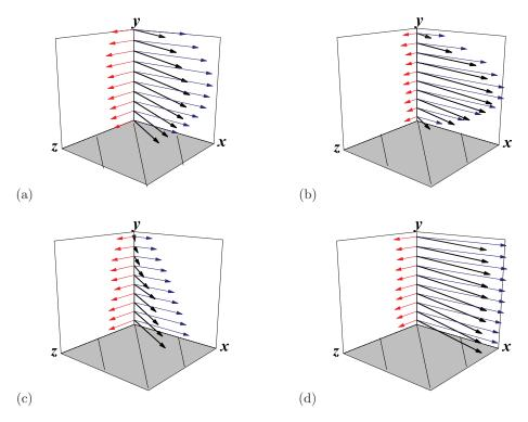
FIG. 10. The velocity profile across the channel at  $\Theta = \pi/4$ , (a)  $H = 10\sigma$ , y from  $-5\sigma$  to  $5\sigma$ , (b)  $H = 50\sigma$ , y from  $-25\sigma$  to  $25\sigma$ , (c)  $H = 50\sigma$ , y from  $15\sigma$  to  $25\sigma$ , enlarged part near the striped-pattern, and (d)  $H = 50\sigma$ , y from  $-5\sigma$  to  $5\sigma$ , enlarged part near the channel center. The z components in (c) and (d) have been increased five times for better demonstration.
