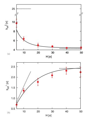
FIG. 8. The longitudinal (a) and transverse (b) effective slip lengths as a function of the channel height *H* for a texture with  $L = b = 50\sigma$  and  $\phi_2 = 0.5$ . The theoretical curves are obtained by a numerical solution of Eqs. (19), (20) and (30), (31). Dashed lines show expected asymptotics in the limit of thin and thick channels.
