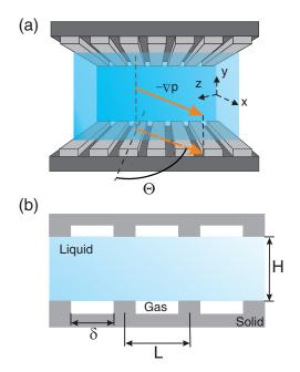
FIG. 1. Sketch of the symmetric striped channel (a)  $\Theta = \pi/2$  corresponds to transverse stripes,  $\Theta = 0$  to longitudinal stripes; (b) situation in (a) is approximated by a periodic cell of size *L*, with equivalent flow boundary conditions on the gas-liquid and solid-liquid interfaces.
