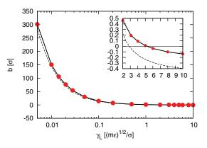
FIG. 2. The relation between the slip length *b* and the wall friction parameter  $\gamma_L$ , for a wall interaction cutoff 2.0 $\sigma$ . The inset shows an enlarged portion of the region where the slip length is zero. The no-slip boundary condition can be implemented by using  $\gamma_L = 5.26\sqrt{m\epsilon}/\sigma$ . Dashed curves show analytical predictions.<sup>37</sup>
