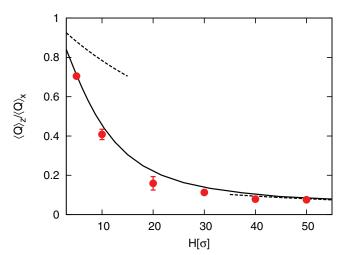
FIG. 9. The ratio between the transverse and longitudinal flow rates  $\langle Q \rangle_z / \langle Q \rangle_x$  as a function of channel thickness *H* for a pattern with  $L = b = 50\sigma$ ,  $\phi_2 = 0.5$ , and  $\Theta = \pi/4$ . Symbols are simulation data and the lines represent theoretical values obtained using Eq. (39). Dashed lines show expected asymptotics in the limit of thin and thick channels.
