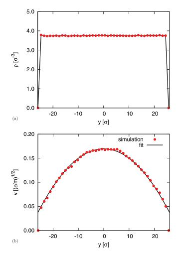
FIG. 3. Typical density (a) and velocity (b) profiles simulated for a longitudinal flow and a texture with  $L = H = b = 50\sigma$ ,  $\phi_2 = 0.5$ .
