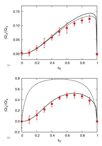
FIG. 7. The ratio  $\langle Q \rangle_z / \langle Q \rangle_x$  as a function of  $\phi_2$  obtained with Eq. (39) for  $\Theta = \pi/4$  by using the data sets from Fig. 6 (a)  $H = 50\sigma$  and (b)  $H = 10\sigma$ . Symbols are simulation data, solid curves represent theoretical values, and dashed curves show asymptotic predictions in the limit of thick channels (a) and thin channels (b).
