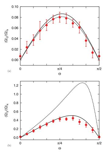
FIG. 5. The ratio  $\langle Q \rangle_z / \langle Q \rangle_x$  as a function of the tilt angle  $\Theta$  obtained with Eq. (39) for the data sets from Fig. 4 for (a)  $H = 50\sigma$  and (b)  $H = 10\sigma$ . Symbols are simulation data, solid curves represent theoretical values, and dashed curves show asymptotic predictions in the limit of thick channels (a) and thin channels (b).
